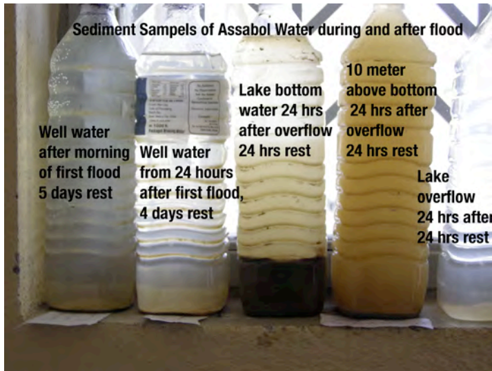
Various water samples revealed a high stratification of lake water, changing within few hours and that the intake water is good enough for pipe flow.
